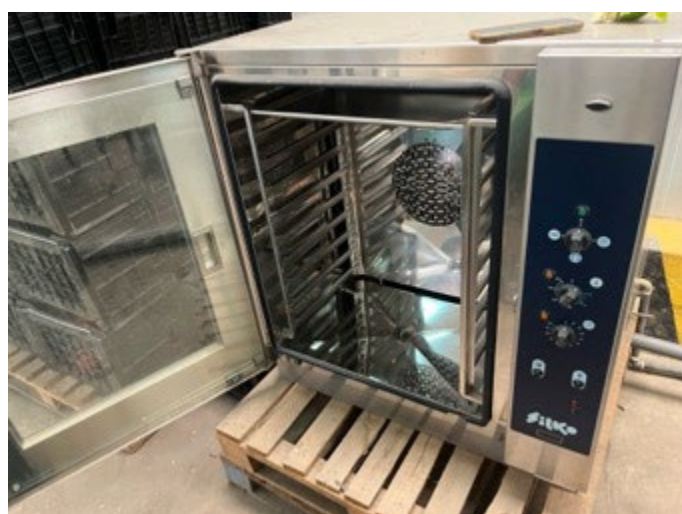
Figure 1: example of a cabinet dryer with a small capacity of approximately 20kg of fresh fruit slices
