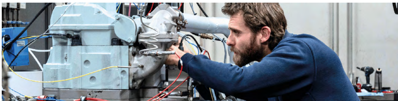
Leading research institute TNO operates a high-tech testing facility for innovations in the powertrains of trucks, including modifications of existing engine platforms to run on new fuels, such as hydrogen, methanol and ammonia.
