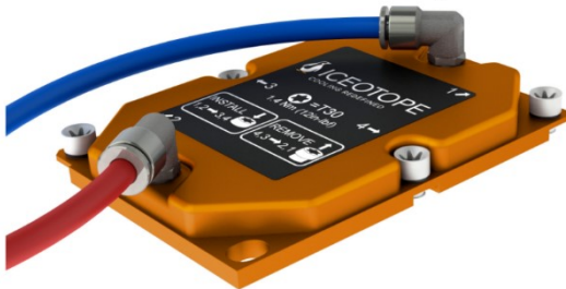
Warm water cold plate cooling
