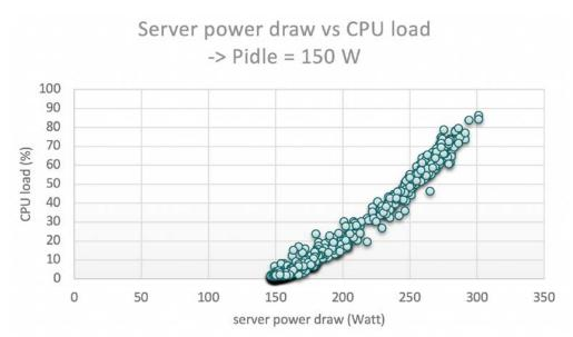
Figure 11: Power vs CPU load
