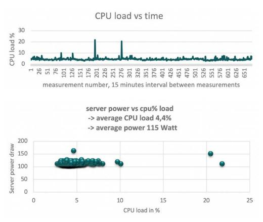
Figure 12: underloaded server configured as "static high performance".
