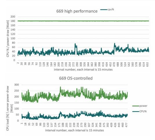
Figure 5: single server configured with static (top) and dynamic (bottom) power. In these graphs, the vertical axis has a double meaning, the CPU load is shown as a percentage from 0% (idle) to 100% (fully loaded), the electrical power draw P of the server is shown in Watt. The horizontal axis just shows the number of the measurement interval.
